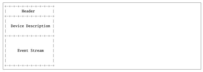
The header contains metadata describing the recording. The device description contains information about input devices involved in this recording. Finally, the event stream contains the recorded input events.
